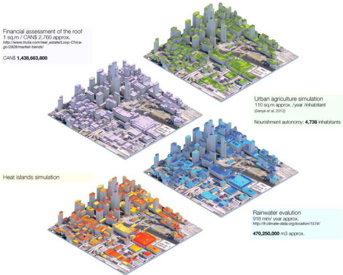
**Figure 2. Roofscape evaluation/simulation**
